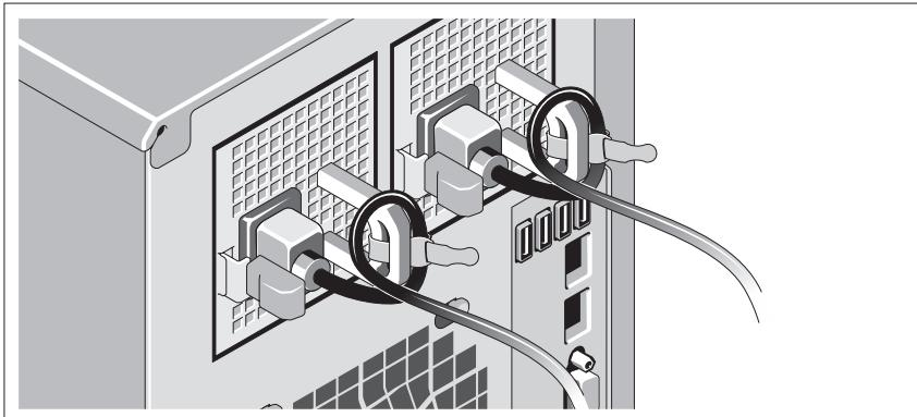
Bend the system power cable(s) into a loop as shown in the illustration and secure the cable(s) with the provided strap.
